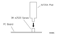
Plug the pod directly into the @3M 2520-series, or similar alternative connector on the PC board.
