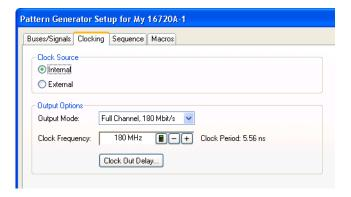
Use an internal clock source when you want to have control over the frequency of the output vectors and it is not important for the output vectors to be synchronized to the system under test.
