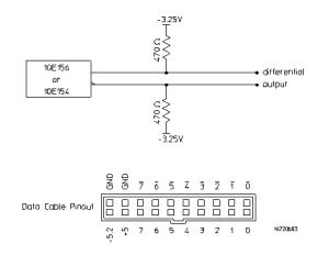
The data cables without a data pod provide an ECL-terminated (470 ohm; to -3.25V) differential signal. These signals are usable when received by a differential receiver, preferably with a 100 ohm termination across the lines. These signals should not be used single-ended due to the slow fall time and shifted voltage threshold; they are not ECL compatible.
